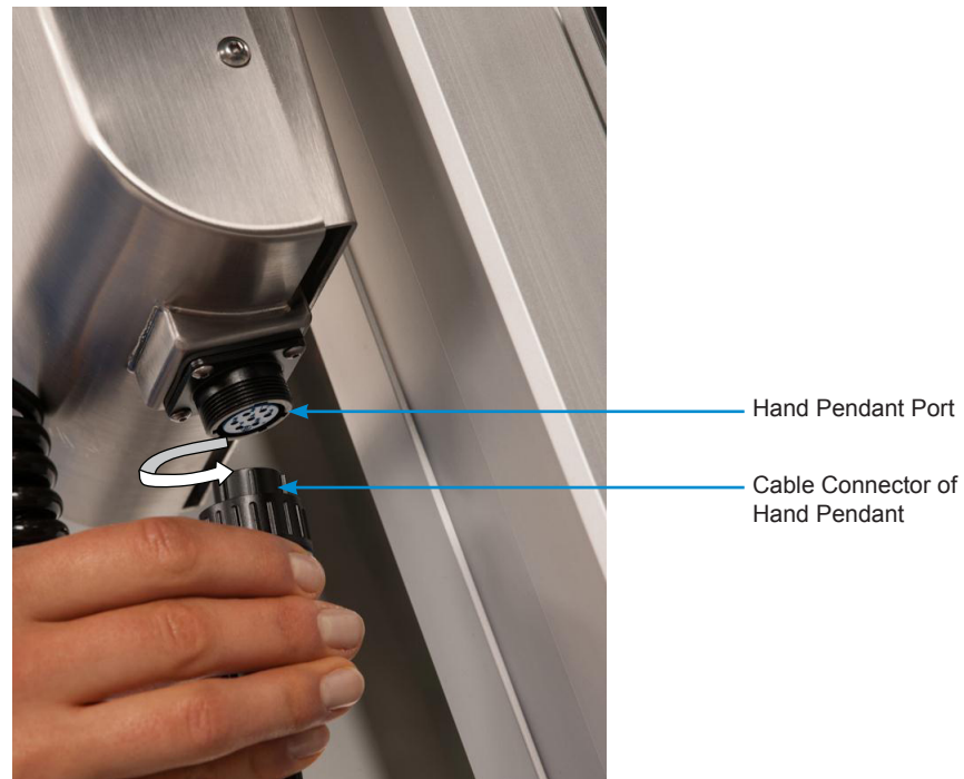
Figure 12: Connecting the Hand Pendant
