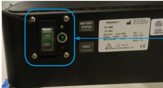
Screws around the Circuit Breaker Plate
