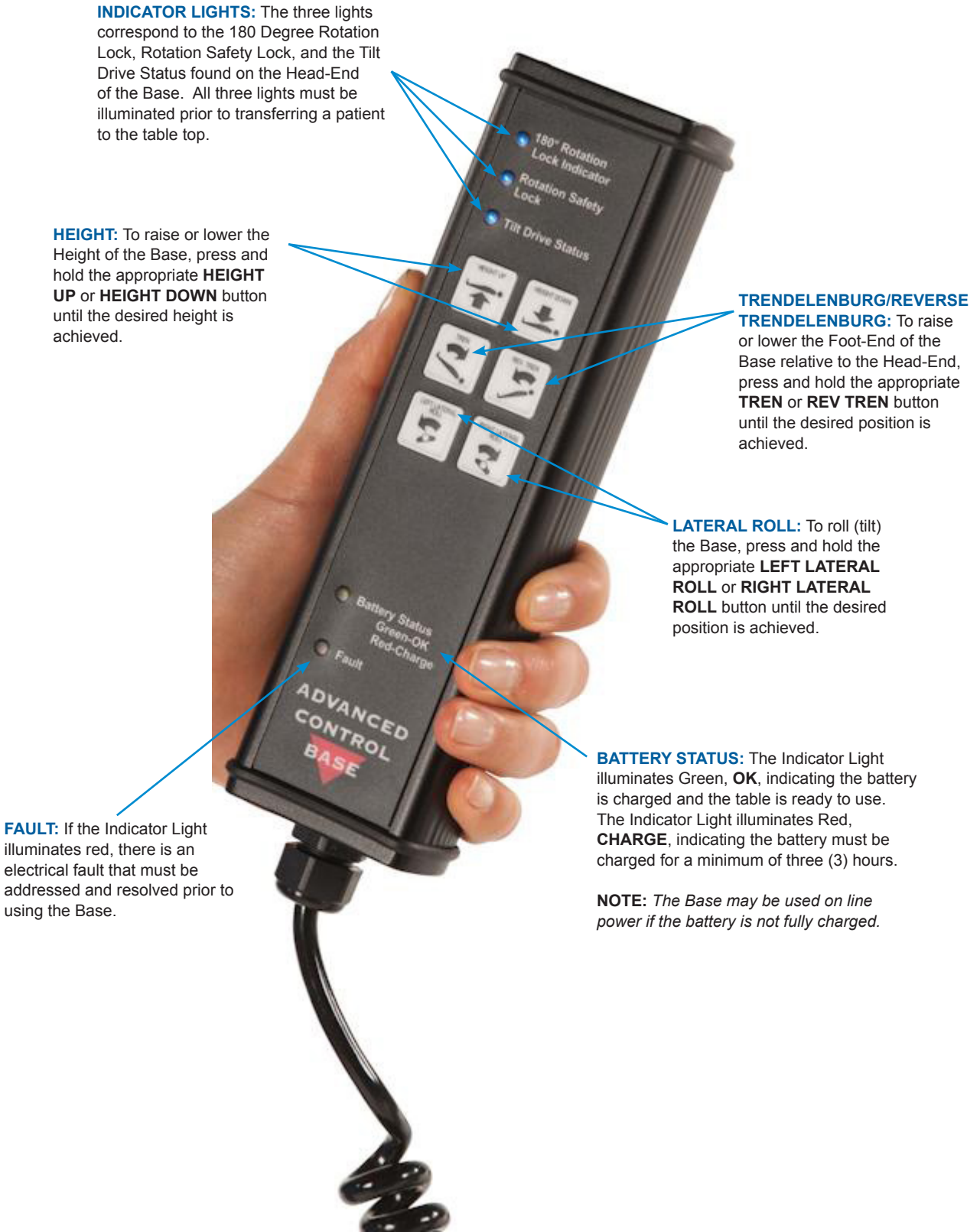
Figure 14: Hand Pendant Functions
