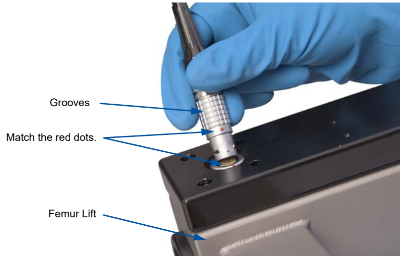
Figure 42: Connecting Coiled Hook Motor Cable to Femur Lift
