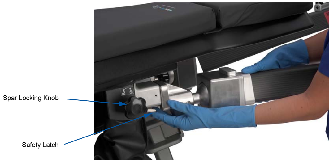
Figure 11: Locking and Unlocking the Leg Spar
